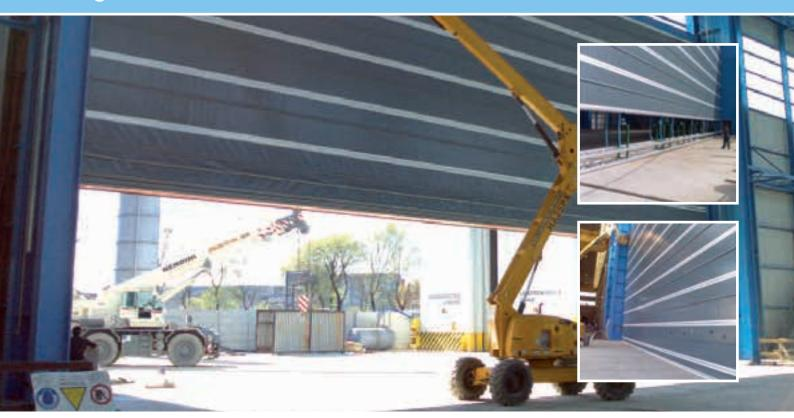
This door is designed for installation internally or externally. Simple free standing, modular design making for a fast and easy installation, depending on the size. The door design consists of a U-shaped column section finished with a rubber seal on each side to protect the curtain whilst operating.
